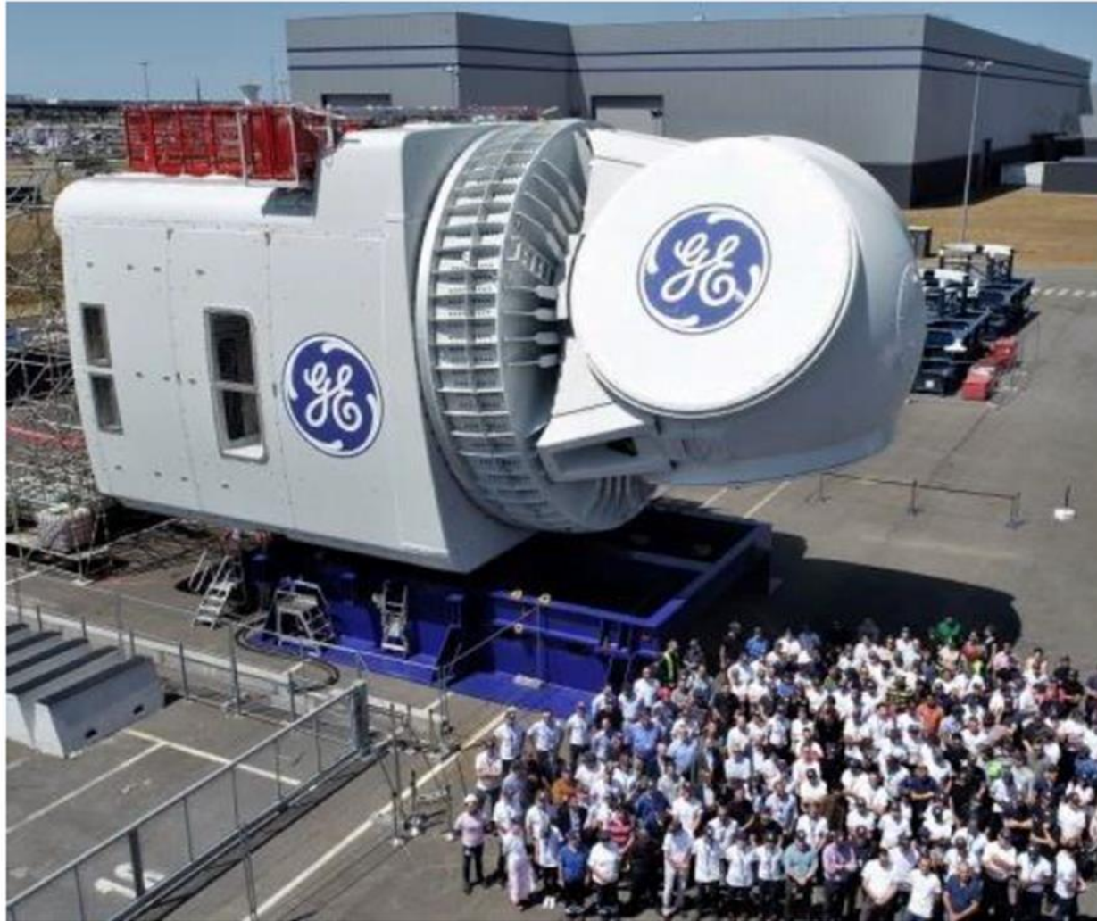
GE Haliade-X nacelle: 13 MW, 220m rotor, ~600 tons
