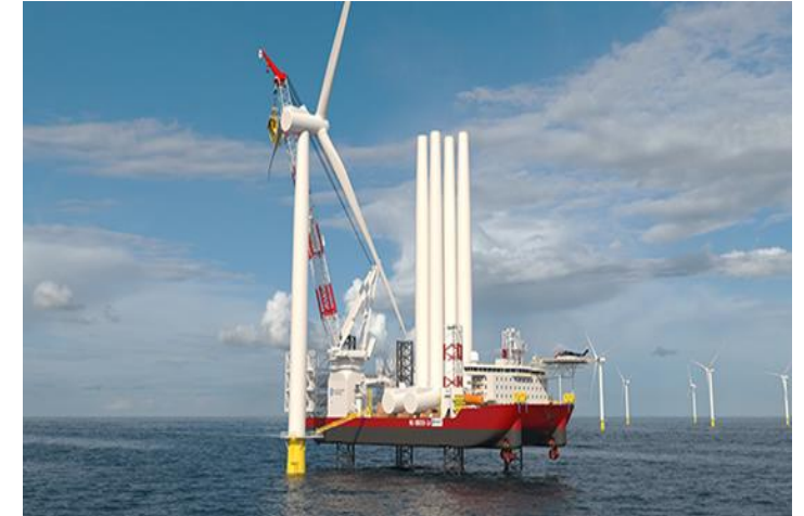
"Charybdis" 1 st Jones Act compliant offshore wind turbine installation vessel
