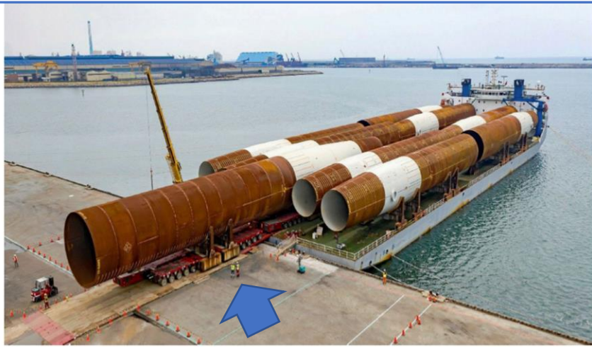
EEW SPC, Monopile load-out for Taiwanese Formosa 1 project in Rostock (GER)
