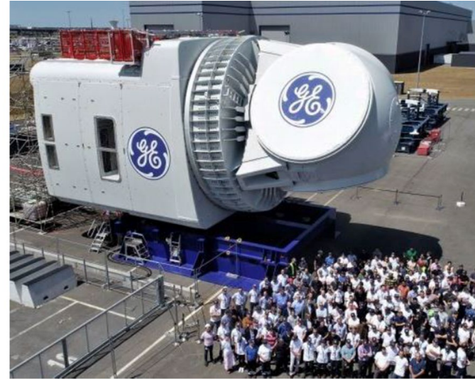
Figure 10 GE Haliade-X nacelle: 13MW, 220m rotor,
