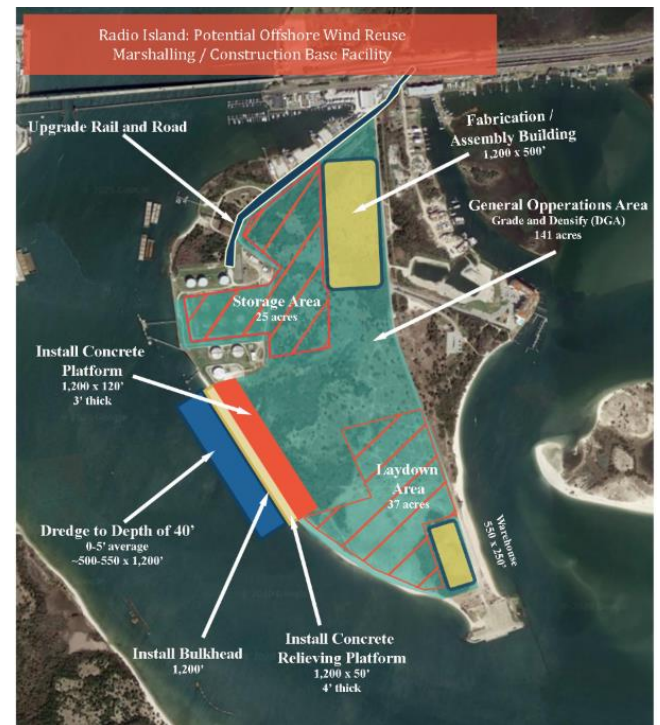
Figure 34 Re-use construction base / marshaling facility scenario for Radio Island.
