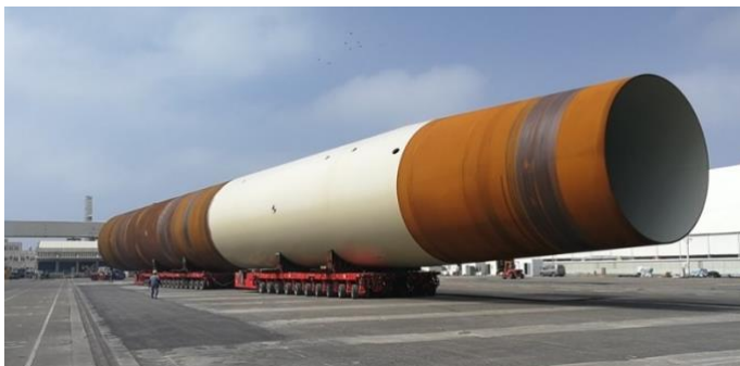
Figure 13 Monopile departs Steelwind Nordenham for Yunlin windfarm: mass 1,732 tons, diameter 8 m, length 93 m.
