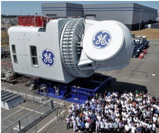
Figure 10 GE Haliade-X nacelle: 13MW, 220m rotor, ≈600 tons.
