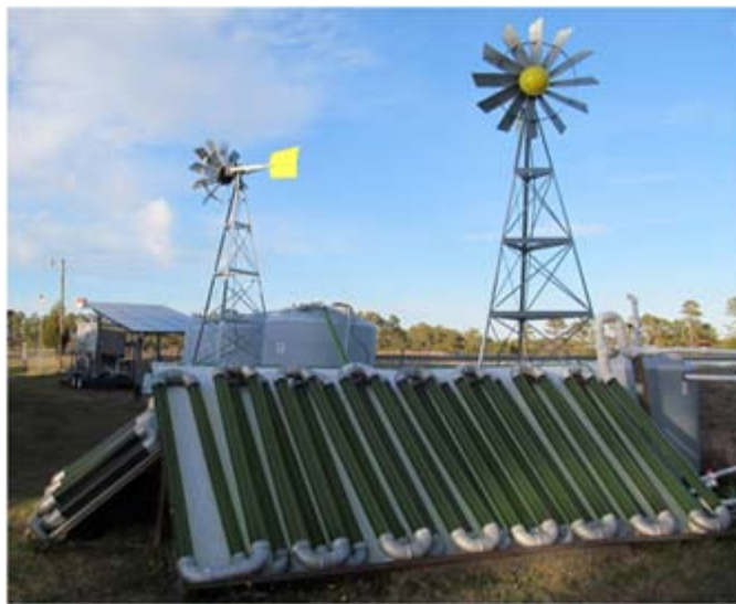
Alganomics' renewable energy generating facility in Southport (photo courtesy of Cape Fear Solar Systems)
