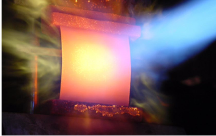
A material used in auto parts undergoes a heat test. The material has been coated with a nanomaterial to enhance its heat resistance. Photo by nCoat
